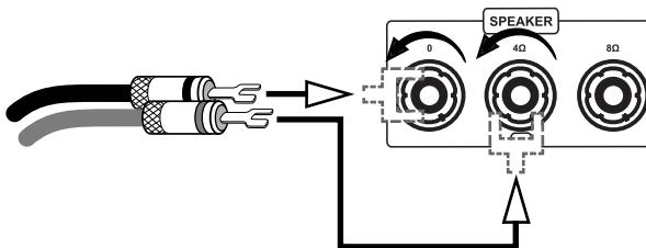
If no connector is to be used, remove approximately 1 cm length of insulation from each end of the speaker wire. Twist the braid in order to avoid short circuits. Turn the fastener on the loudspeaker terminal counter clockwise to loosen it and introduce the bare wire end into the exposed connector hole. Then turn the fastener clockwise so that the wire is firmly clamped. Make sure the connection is pretty tight.
